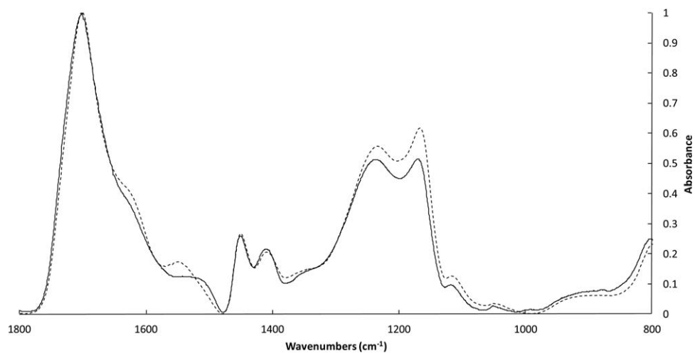
Figure 5. The FTIR spectrum of electrospun 8% poly(acrylic acid)/0.8% lysine before heating (dashed line) and after heating (solid line).
